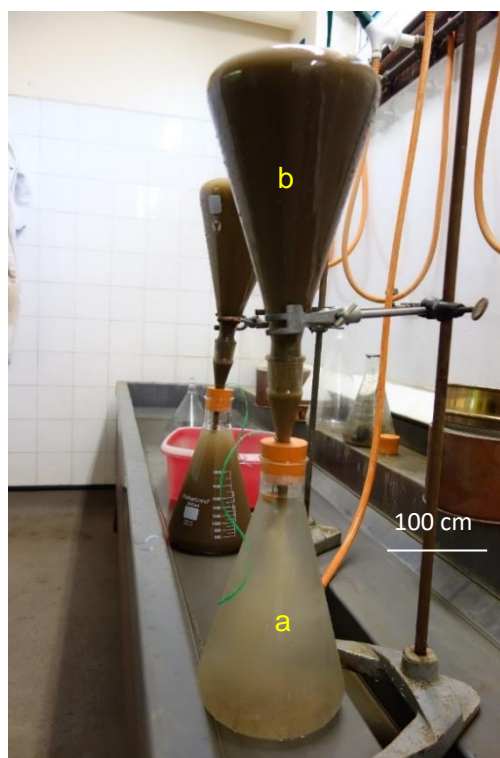
Figure 2.3. Seinhorst two-flask method showing the sedimentation process. Soil particles with more density than nematodes are collected in flask (a) while nematodes remain in flask (b)
