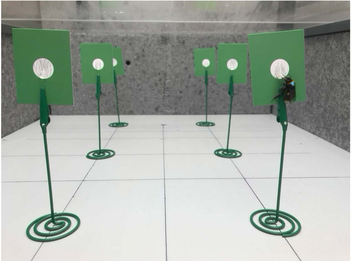
Figure 2.11 Setup for printed models in differential conditioning experiments. Three of each model type were placed in an equally spaced alternating array inside the arena. One type of model (e.g. Maris Bead vein pattern) were loaded with 10 \mu l of 40% w/w sugar solution and the other (e.g. NV129 vein pattern) were loaded with quinine hemisulphate solution (0.12% w/w) as a punishment. The first 100 drinking visits made by a bee were recorded. When a bee was full and returned to the colony box models were then replaced with new models to eliminate any scent marks and the orientation was swapped to eliminate positional effects. Responses of five bees were recorded when model type A was rewarded (e.g. Maris Bead vein pattern) and responses of five bees were recorded when model type B was rewarded (e.g. NV129 vein pattern).
